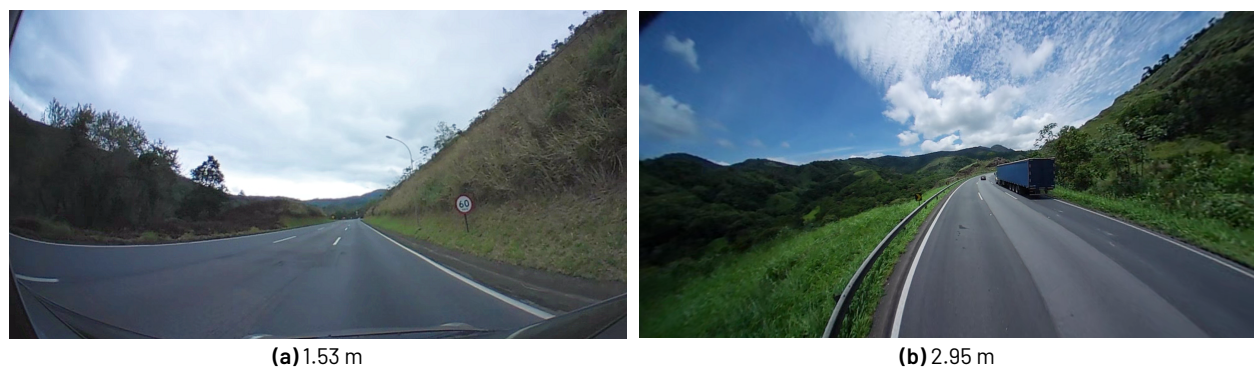
Figure 3 • Photographs illustrating the two camera heights used during the evaluation. (a) 1.53 m; (b) 2.95 m.
