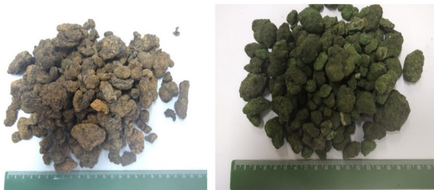
Figure 1. Asphalt rubber pellet samples used in this study - PelletPAVE-Plus (left) and PelletPAV (right)
